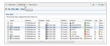
Keep in mind that the first rule in the Tofino SA that matches is applied to the packet: not the rule that is the most appropriate match. Based on this, set the more specific rules at the top of the list, followed by the more general rules. This helps to prevent a general rule being matched before hitting a more specific rule.
