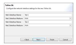
Name the Tofino SA interfaces and set the configuration of each interface.
