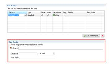
You can adjust advanced settings, such as traffic rate limiting, for most rule profiles. Additional settings for the selected rule profile are displayed in one or more tabs below the table.
